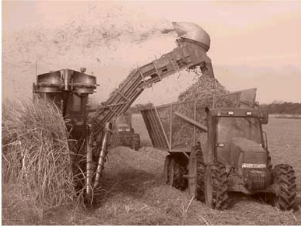
Figure 4.25. Sugarcane Billet harvester. Photo by Douglas Durand, Jr., Louisiana State University Agricultural Extension Service. Used by permission.
