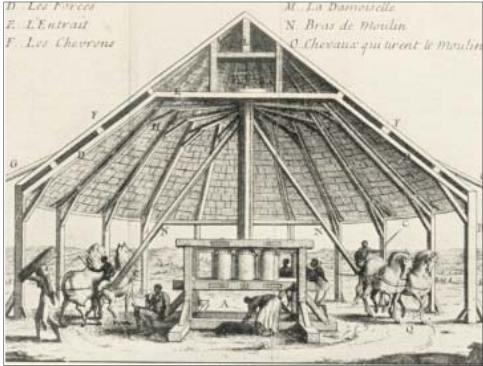
Figure 3.10. Animal-Powered Three-Roller Sugar Mill. The three-roller mill was an Arab improvement on the Indian vertical, two-roller mill. This innovation was used for centuries in the Mediterranean, the East Atlantic sugar islands, Brazil, and the Caribbean. Source: Noel Deerr, The History of Sugar (London, 1949), Plate 27, facing p. 230.
